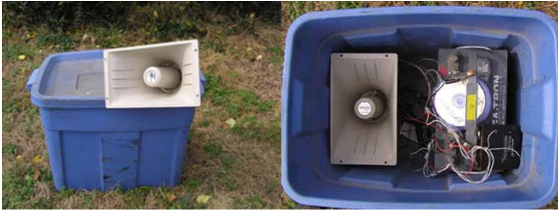
Photos of audio lure components. Photo on left shows components inside plastic container including battery, CD player, amplifier, and bell speaker and connectors. Photo on right shows audio lure in operation with external bell speaker. Photos by Fletcher Smith.
